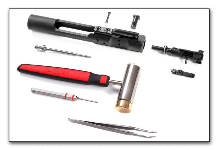
These are the simple main tools necessary for the standard disassembly of an AR platform
