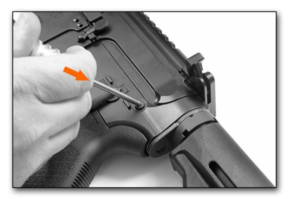
Push the two pins that lock  $\underline{\text{\bf upper and lower}}$
