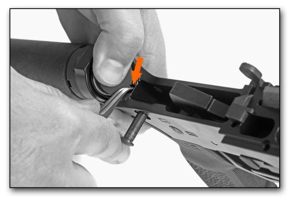
Holding the  $\underline{\text{buffer}}$  still and using a suitable tool, press down the spring lock pin
