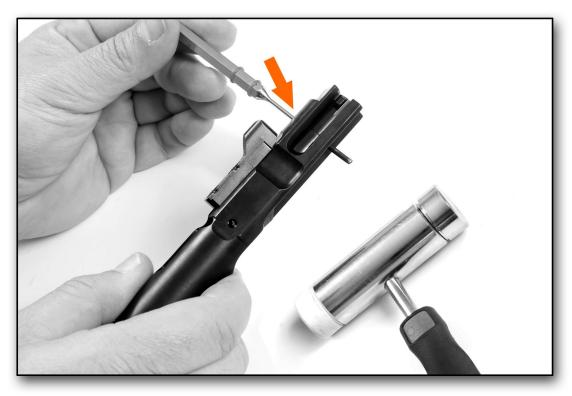
With a pin-chaser, push out the  $\underline{\text{pin}}$  that blocks the  $\underline{\text{extractor}}$
