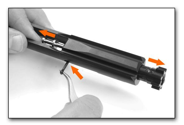
Withdraw the  $\underline{\text{pin}}$  completely and release the  $\underline{\text{firing pin}}$  with its spring. Move the bolt completely back
