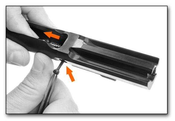
Withdraw the pin completely and release the firing pin with its spring
