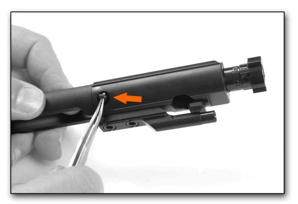
Remove the firing pin locking pin with the help of a tool
