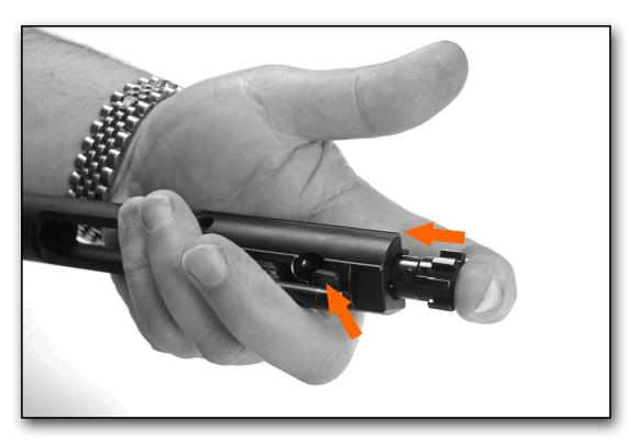
Now push the <u>bolt</u> back into the carrier (the <u>cam</u> now positions itself forward for the extraction phase)
