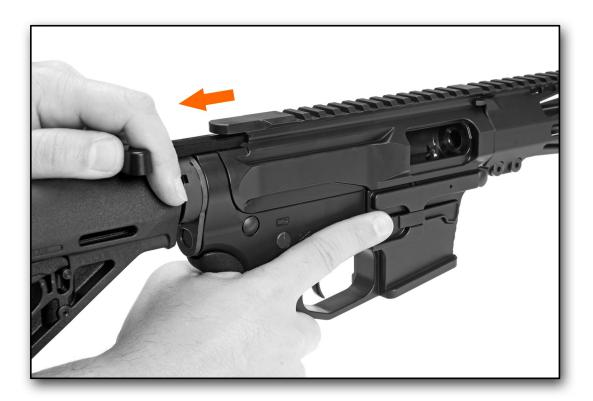
Move the cocking lever back until the bolt locks in the open position
