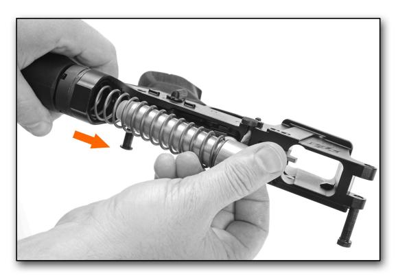
Now carefully extract all the  $\underline{\text{spring}}$  and the  $\underline{\text{buffer recoil}}$  from the tube
