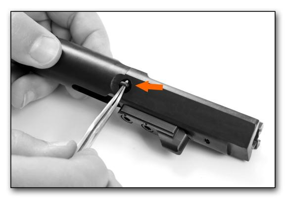
Remove the locking pin of the firing pin with the help of a tool
